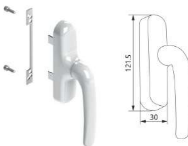
WH-23 Material: Zinc alloy bottom+Aluminum alloy handle Finish: Powder coating, Oil injection Colour: Black, White, Silver, Brown, Beige
