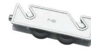
WW-15-D (P-92) Material: Zinc alloy Finish: Electroplating blue zinc Wheel Size: \Phi 28mm Bearing: 60kg
