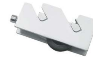
WW-15 (P-92) Material: Zinc alloy Finish: Electroplating blue zinc Wheel Size: \Phi 28mm Bearing: 30kg
