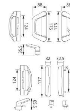
SDH-06 Material: Aluminum alloy + Zinc alloy Finish: Powder coating, Oil injection Colour: Black, White, Silver
