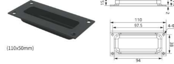
SDH-24-1 Material: Aluminum Finish: Powder coating, Oil injection Colour: Black, White, Silver
