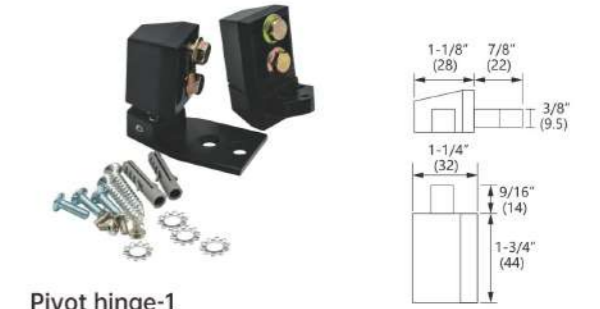
Pivot hinge-1 Material: Aluminum alloy Finish: Powder coating, Oil injection, Oxidation Colour: Black, White, Silver, Grey, Beige
