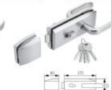
GDL-06 Material: Aluminium alloy with stainless steel plate Suited door thickness: 8-12mm Finishing: Satin/polish/black
