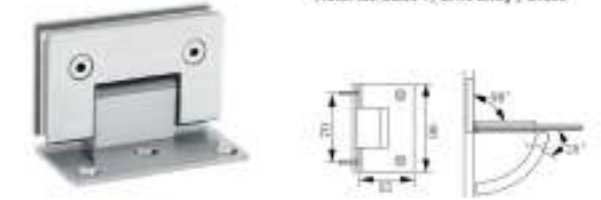
SH-008(90° , one side) Material: SS304 / Zinc alloy / Brass
