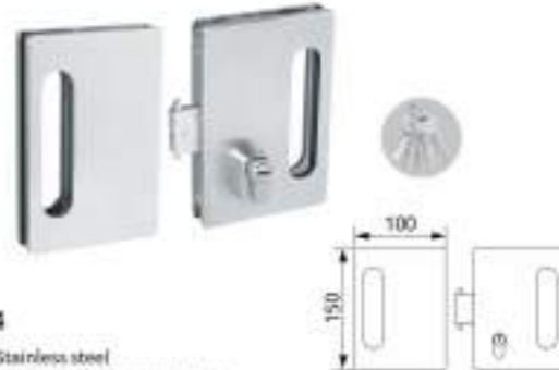
GDL-12 Material: Stainless steel Suitable for 10-15mm tempered glass Finishing: Satin/polish/black
