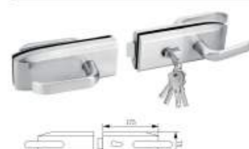
GDL-05 Material: Aluminium alloy with stainless steel plate Suited door thickness: 8-12mm Finishing: Satin/polish/black
