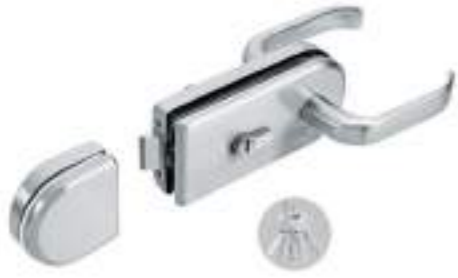
GDL-11 Material: Stainless steel Suitable for 10-15mm tempered glass Finishing: Satin/polish/black
