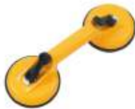
ST-05 Level suction: 90kg Vertical suction: 75kg Material: Aluminium alloy
